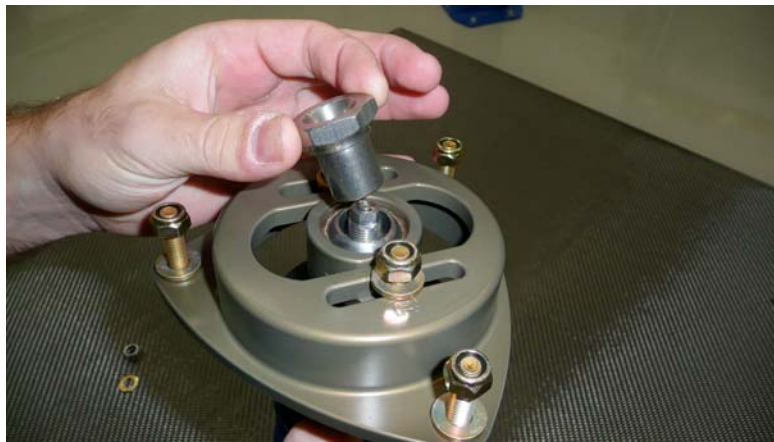
RCE Camber Plate installed and centered on top of RCE Washer
