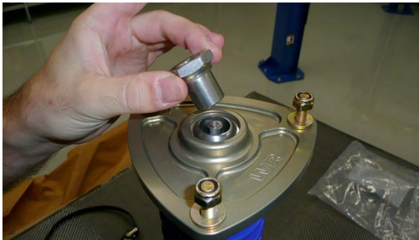
Rear RCE Pillowball Mount installed and centered on top of washer.
