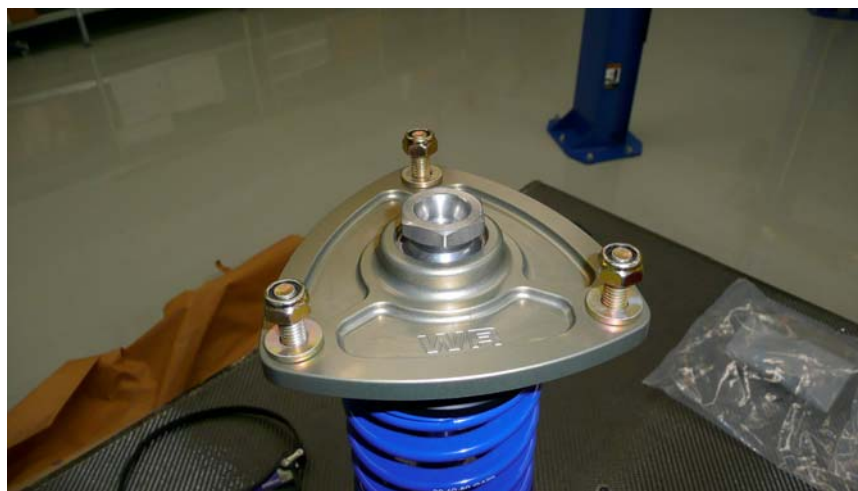
Rear Pillowball Mount installed with inset top nut. Torque top nut to 30 ft-lbs. Use a strap wrench to prevent shaft from spinning.
