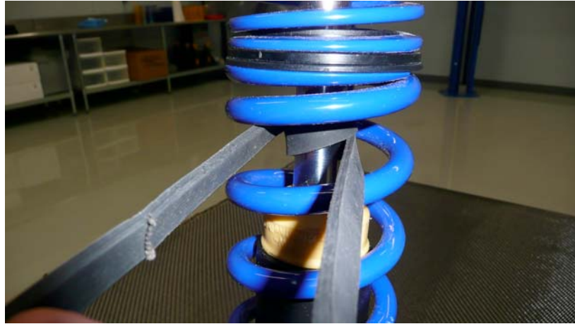
Strap wrench wrapped twice around strut shaft.
