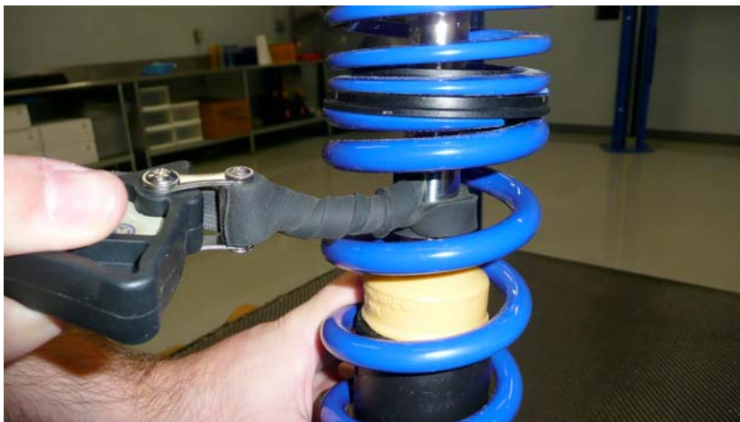
Strap wrench twisted and held tightly. Now torque top nut to 30 ft-lbs.
