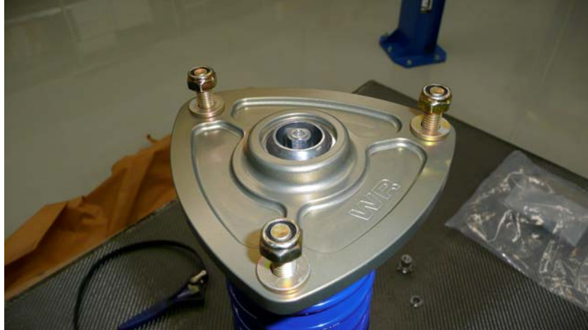
Rear RCE Pillowball Mount installed and centered on top of washer.
