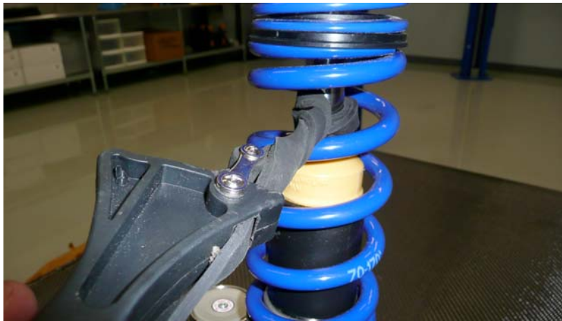
Strap wrench wrapped twice around strut shaft.
